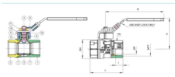
The Buna O-ring is fitted to the stem of the valve as the best possible protection against potential gas leakage under extreme duty, or low pressure applications. A secondary P.T.F.E stem seal will also assure that the valve is suitable for use up to 366°F.
