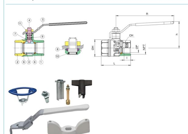
The NBR O-ring is fitted to the stem of the valve as the best possible protection against potential gas leakage under extreme duty, or low pressure applications. A secondary FKM (Viton) stem O-ring seal will also assure that the valve is suitable for use up to 366°F.
