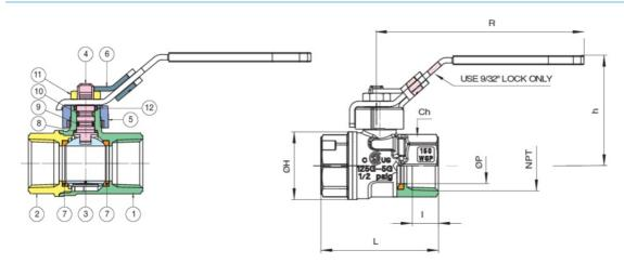
The Buna O-ring is fitted to the stem of the valve as the best possible protection against potential gas leakage under extreme duty, or low pressure applications. A secondary PTFE stem seal will also assure that the valve is suitable for use up to 366°F.
