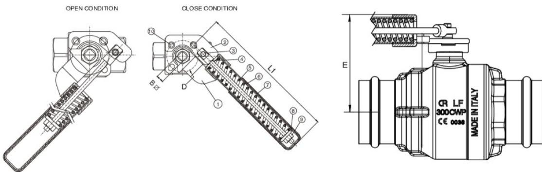
The Buna O-ring is fitted to the stem of the valve as the best possible protection against potential gas leakage under extreme duty, or low pressure applications. A secondary P.T.F.E stem seal will also assure that the valve is suitable for use up to 366°F.
