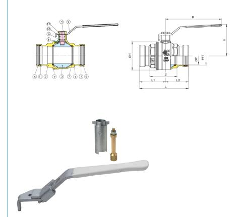
The NBR O-ring is fitted to the stem of the valve as the best possible protection against potential gas leakage under extreme duty, or low pressure applications. A secondary FKM (Viton) stem O-ring seal will also assure that the valve is suitable for use up to 366°F.
