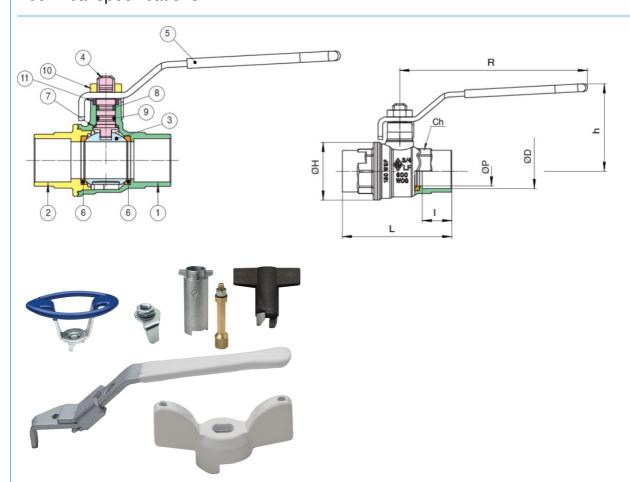
The Buna O-ring is fitted to the stem of the valve as the best possible protection against potential gas leakage under extreme duty, or low pressure applications. A secondary P.T.F.E stem seal will also assure that the valve is suitable for use up to 366°F.
