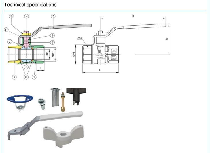
The NBR O-ring is fitted to the stem of the valve as the best possible protection against potential gas leakage under extreme duty, or low pressure applications. A secondary FKM (Viton) stem O-ring seal will also assure that the valve is suitable for use up to 366°F.
