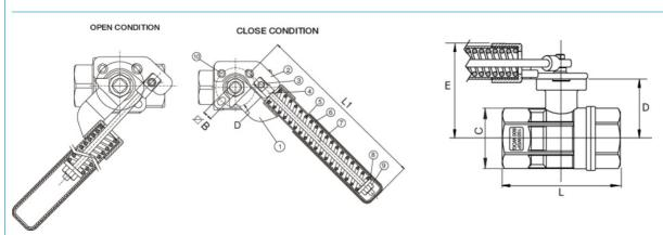
The Buna O-ring is fitted to the stem of the valve as the best possible protection against potential gas leakage underextreme duty or low pressure applications.
