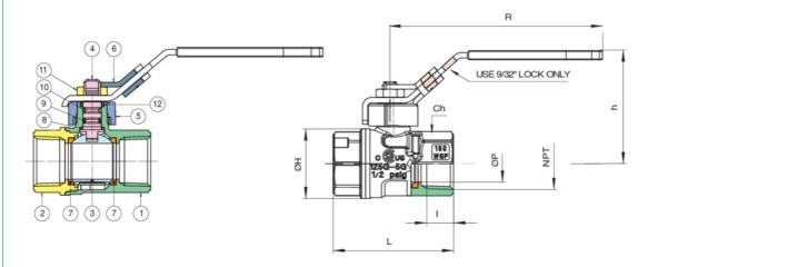
The Buna O-ring is fitted to the stem of the valve as the best possible protection against potential gas leakage under extreme duty, or low pressure applications. A secondary PTFE stem seal will also assure that the valve is suitable for use up to 366°F.
