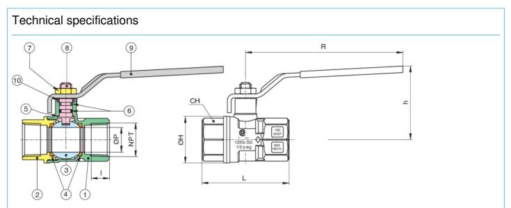
The NBR O-ring is fitted to the stem of the valve as the best possible protection against potential gas leakage under extreme duty, or low pressure applications. A secondary FKM (Viton) stem O-ring seal will also assure that the valve is suitable for use up to 366°F.
